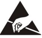
Electrostatic discharge can affect electronic components. Take precautions to neutralize electrostatic charge by touching your hand and tools to metal prior to handling the control.
