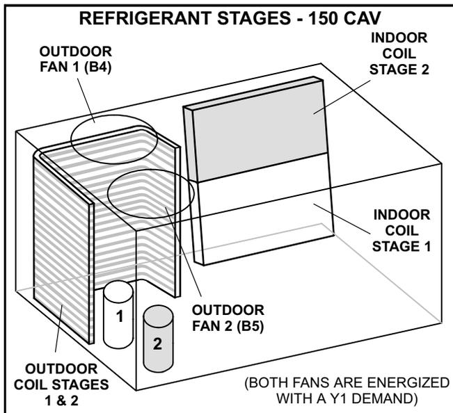
This unit is factory charged and should require no further adjustment. If the system requires additional refrigerant, reclaim the charge, evacuate the system, and add required nameplate charge.
